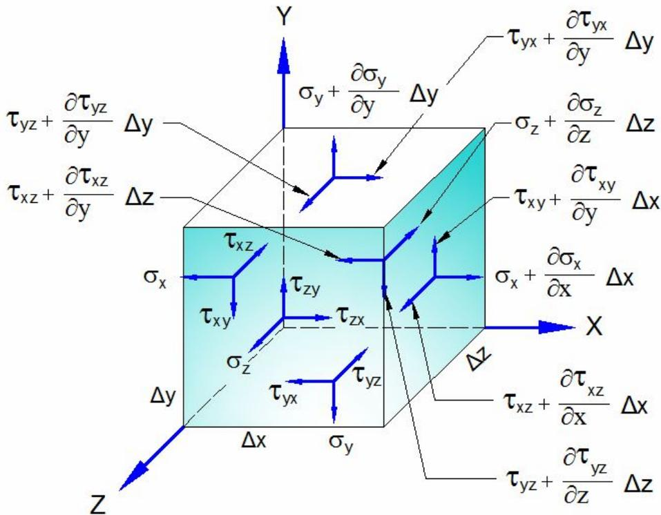
Figure 2.11(b) Stress components acting on a three dimensional element
