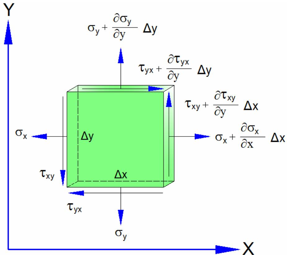
Figure 2.11(a) Stress components acting on a plane element
