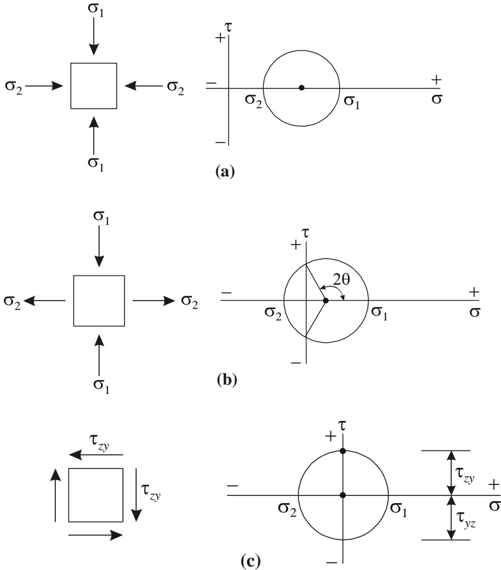
**Figure 2.13 Simple Biaxial stress systems: (a) compression, (b) tension/compression, (c) pure shear**
