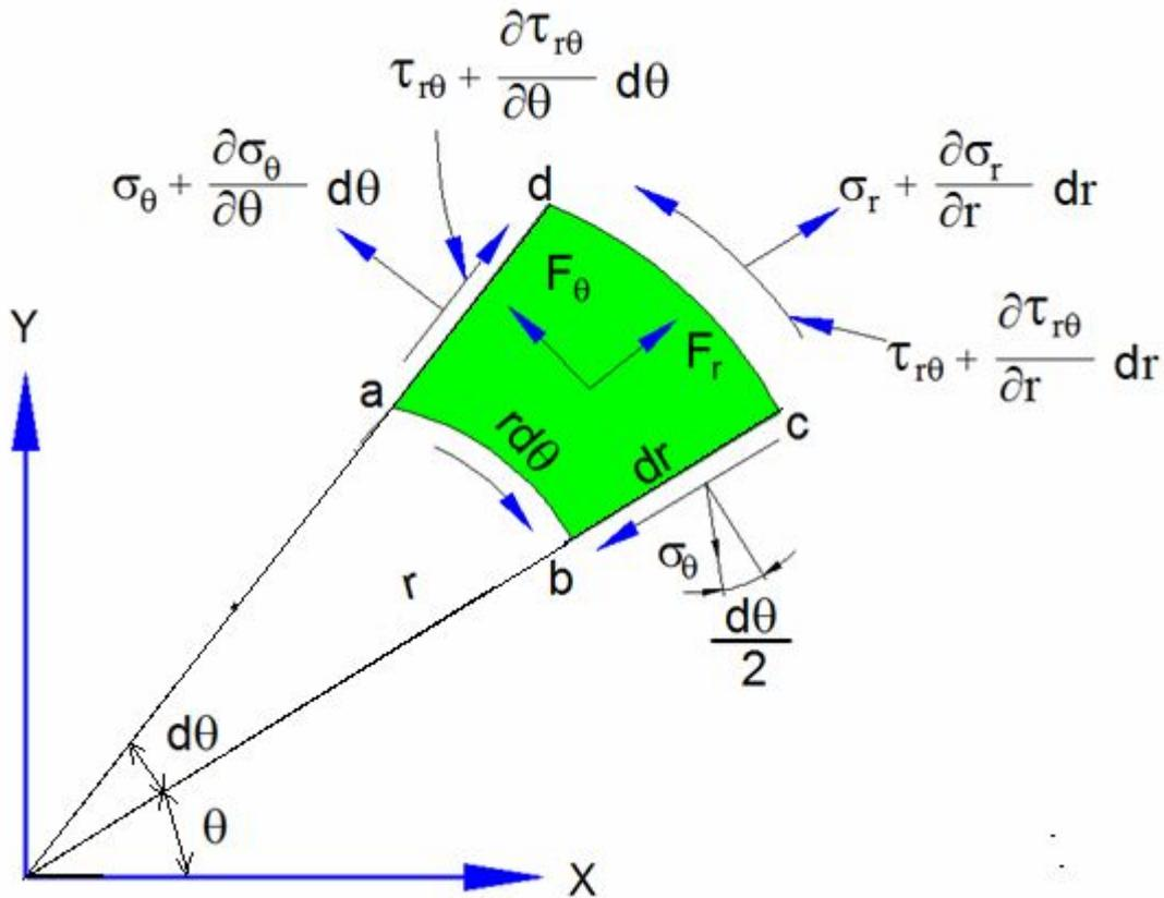
**Figure 2.16 Stresses acting on an element**
