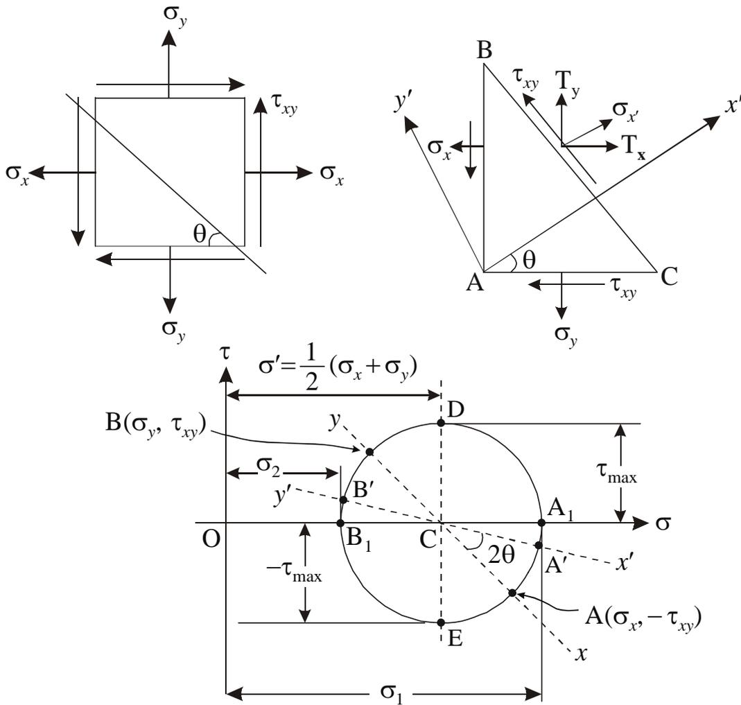
**Figure 2.14 Construction of Mohr's circle**
